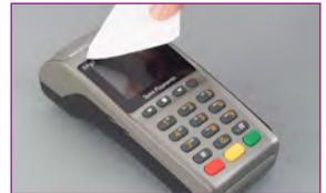
2. With the terminal face down remove the battery cover and battery. Remove the battery packaging. Insert your SIM (sent separately) into the slot marked **SIM1 SLOT**. Insert the battery in to the terminal and replace the cover.
