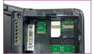
2. Slide the SIM with the chip facing down and the cut corner bottom left underneath the metal bar in the slot marked SIM2 or SIM.
